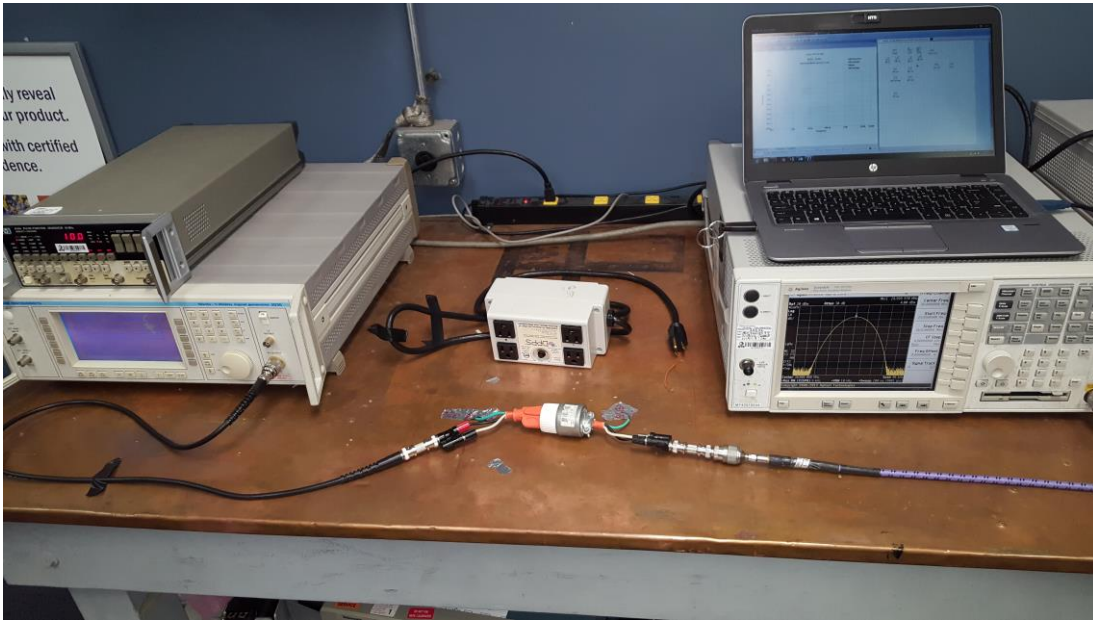
Figure 5-9 Differential Mode Insertion Loss Calibration Setup
